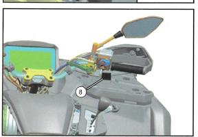
Place heat shrink tubing (8) over the heating band and the throttle switch, heat molding with a hot air gun. After the installation, follow the above steps to restore the vehicle.
