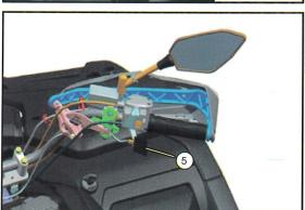
Place heat shrink tubing (5) over the heating band and the throttle switch, heat molding with a hot air gun. After the installation, follow the above steps to restore the vehicle.
