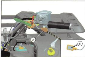
Paste the 3M double-side tape (6) to the heating band (A), then paste the heating band to the throttle switch.
