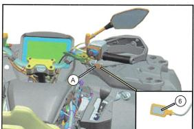
Paste the 3M double-side glue (6) to the heating band (A), then paste the heating band to the throttle switch.
