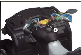
// Remove the steering handlebar cover (A).
