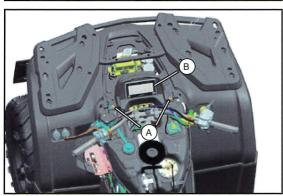
Remove the fixed bolts (A) from dashboard guard, place the dashboard assembly (B) aside.
