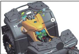
// Remove the fuel tank panel kit (A).
