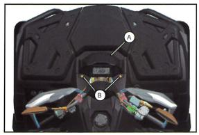
Remove the expansion rivet (B), disassemble the dashboard guard kit (A).
