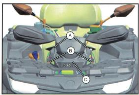
Remove the fixed bolts (A) & (B), and take out the front guard (C) from the dashboard.
