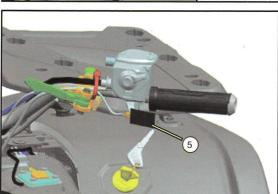
// Place heat shrink tubing (5) over the heating pad and the throttle switch, heat molding with a hot air gun. After the installation, follow the above steps to restore the vehicle.
