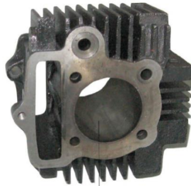
inner cylinder wall
