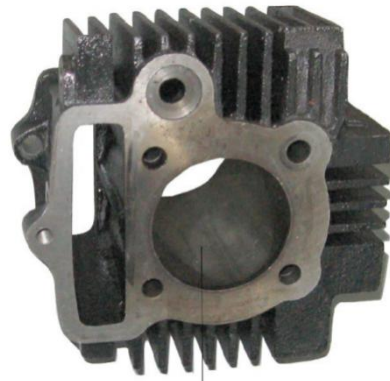
inner cylinder wall
